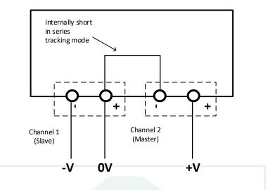
Fig 2. Series tracking mode and duel rail connection
