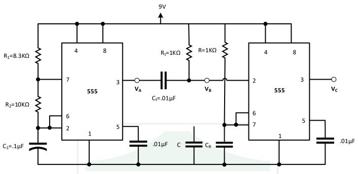
Fig 5: Circuit for capacitance measurement
