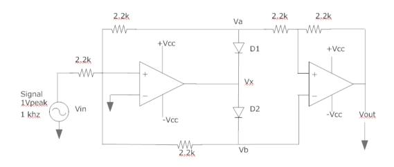
**Fig:Precision full wave rectification**
