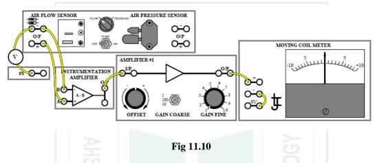
Connect the circuit as shown in Fig 11.10 and set the GAIN COARSE control of Amplifier #1 to 10 and GAIN FINE control to 1.0. Check that the pump control is set to OFF.
