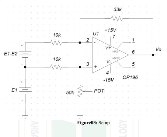
4. Vary the  $(E_1-E_2)$  from 0V to 6V with a step of 0.5 V and measure V<sub>0</sub>. Record the data in the following table.
