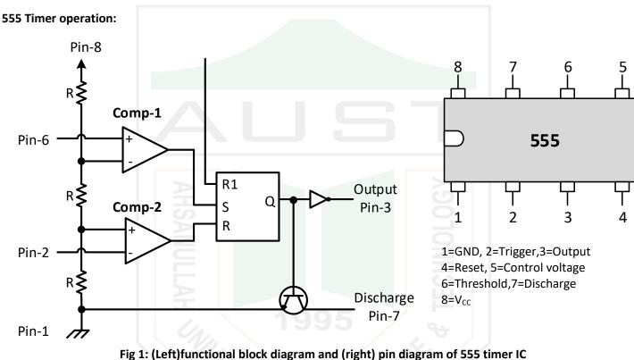
A 555-timer's operation can be modeled using op-amp (used as comparators), SR flipflop, NPN transistor and three equal value resistances as shown in Fig 1.
