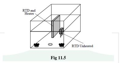
Fig 11.5 shows the construction of an Air Flow Transducer, consisting of two RTD's (Resistance Temperature Dependent) mounted in a plastic case. One of the devices has an integral heating element incorporated with it and the other is unheated.
