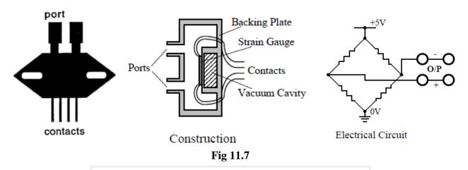
The air pressure in the outer container will produce an output from the bridge and variation of the pressure will produce a variation of this output. The transducer output can be calibrated and may be called an absolute pressure transducer. Provision is made for air to be fed to the unit from the pump.
