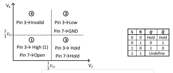
Fig 2: (Left) Operational state of the timer (Right) Truth table of SR flipflop
