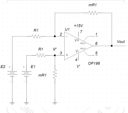
Figure 01: basic differential amplifier
