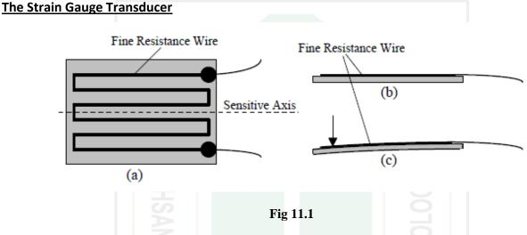
Fig 11.1 shows the construction of a strain gauge, consisting of a grid of fine wire or semiconductor material bonded to a backing material. When in use, the unit is glued to the beam under test and is arranged so that the variation in length under loaded conditions is along the gauge sensitive axis (Fig 11.1(a)). Loading the beam increases the length of the gauge wire and also reduces its cross-sectional area (Fig 11.1(c)). Both of these effects will increase the resistance of the wire.
